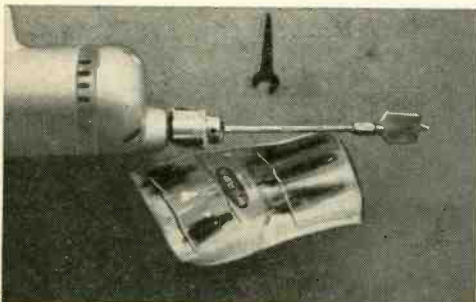
Wood bit in chuck of electric drill. This is not the type bit used with a hand brace.
