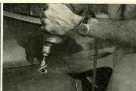
Fly-cutter being used to cut 1-inch hole in car fender for mounting auto-radio antenna.
